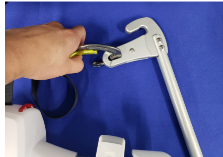
Closed carabiner attached to latch of the Reacher Bar.
