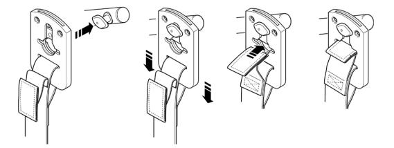
Securi3 sling attachment system. Example of installation.
