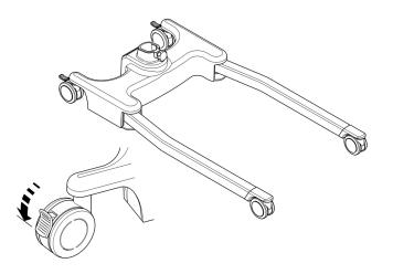
2. Fit the mast and boom assembly into the chassis socket.
