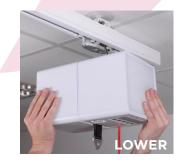
Detachment from the rail takes a matter of seconds. Simply disconnect the charge lead on top of the lift motor and lift, twist and lower the CX12 from its trolley. Attachment is in reverse sequence; remember to connect the charge lead to finish.
