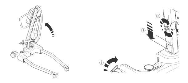
5. Open legs fully. ENSURE leg-locking knob engages flush against the base casting and the legs will no longer move freely. The legs will then only operate by the use of the foot pedal mechanism located at the rear of the base.
