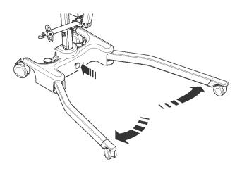
6. Release the spreader bar from the retaining cradle. The lift is now ready for operation.
