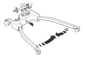
3. Loosen the mast locking device sufficiently to allow the mast to be lifted upwards. Lift the mast fully until the upper stop is reached. Carefully fold the mast towards the legs. Use the push handle to assist this action.
