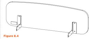
10. Fix the brackets to the footboard using the M8 x 35 bolts, nuts, and washers provided as shown in Figure 8.5. Tighten using the 5mm Allen key and a 13mm spanner.
