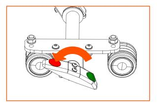
2. To unlock the brake, press firmly downwards on the side of the pedal with the green label as shown in Figure 14.4 until the brake releases.
